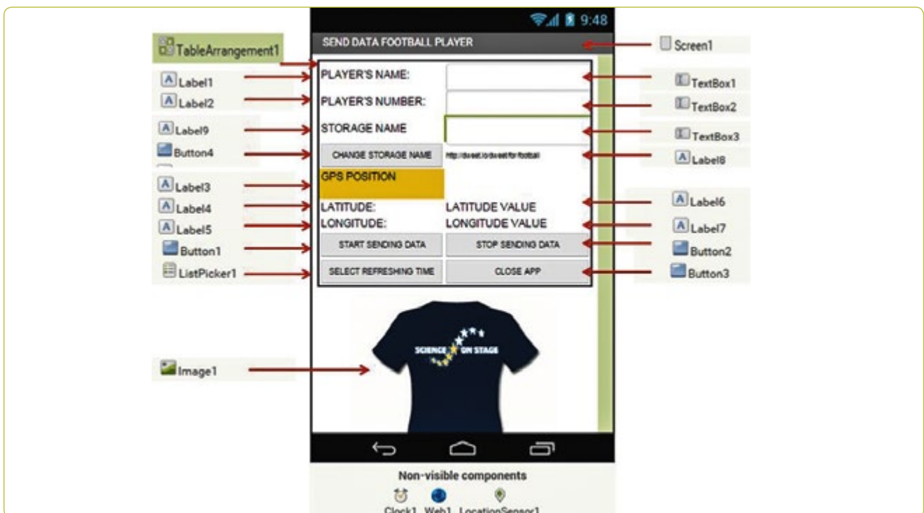
FIG. 2 Components of TableArrangement1
