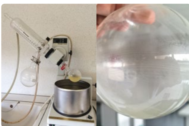
FIG. 8 Evaporation of the solvent using a rotary evaporator (left) · Powder on the side of the flask after the evaporation of the solvent
