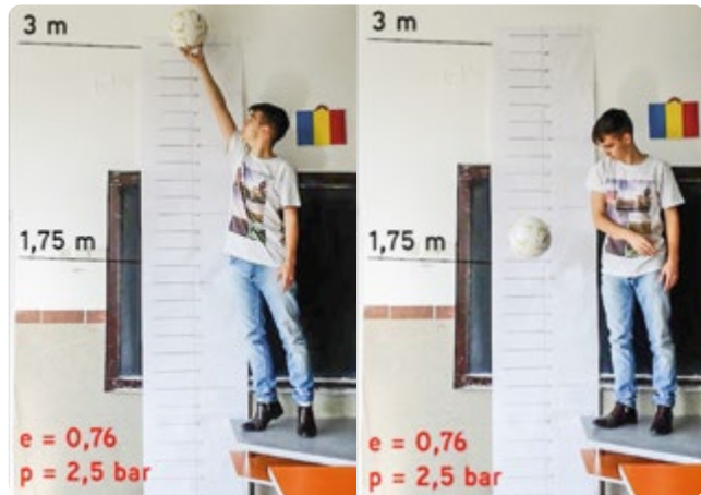
FIG. 5 Hold the ball at the height h_1 (left); drop the ball (right)
